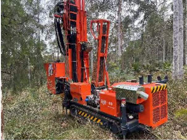
Photo 5: Hanjin D&B 8D drilling rig used for borehole drilling in the Phase 1 development area.
