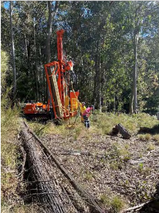
Photo 3: Hanjin D&B 8D drilling rig setup in the Phase 1 development area at BH11.
